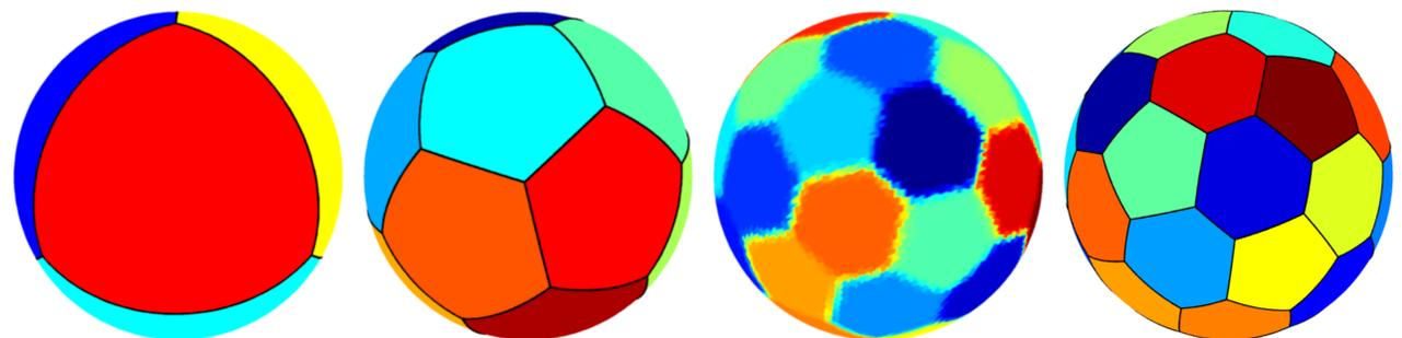
Numerical results (left to right):  $N = 4$ : regular tetrahedron partition,  $N = 12$ : regular pentagons tessellation,  $N = 32$ : density method and refined method. For  $N = 32$  we find the  $C_{60}$  fullerene structure (like a soccer ball: 12 regular pentagons and 20 equal hexagons)
