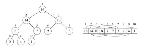
A heap can be represented in a compact way through an array A:
