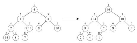
• The initial array is interpreted as a complete binary tree
